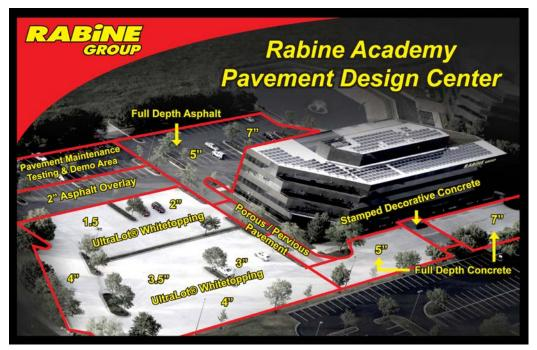
research and development. The parking lot includes, full depth asphalt, full depth concrete, asphalt overlays, UltraLot® Whitetopping, porous asphalt, pervious concrete, stamped concrete, and roller compacted concrete.
